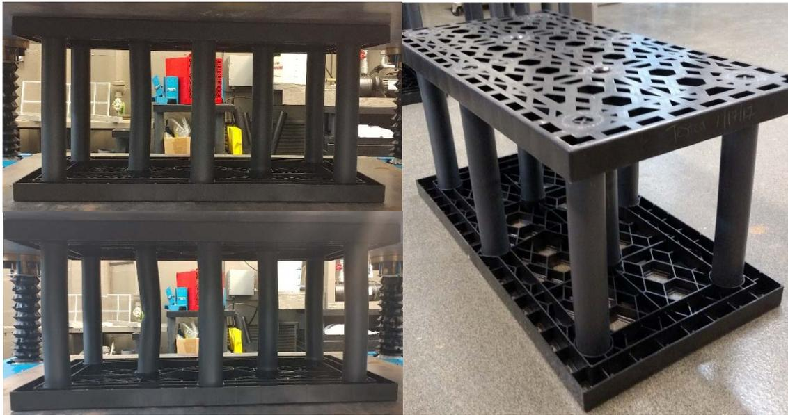
*Figure 1 - 18" Module at 20,000 lbs., at completion, and after removal from steel press*
