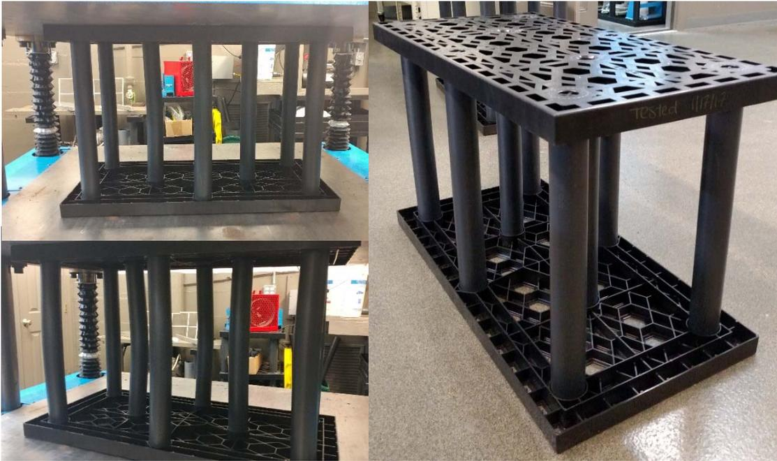
Figure 3 - 24" Module at 20,000 lbs., at completion, and after removal from steel press
