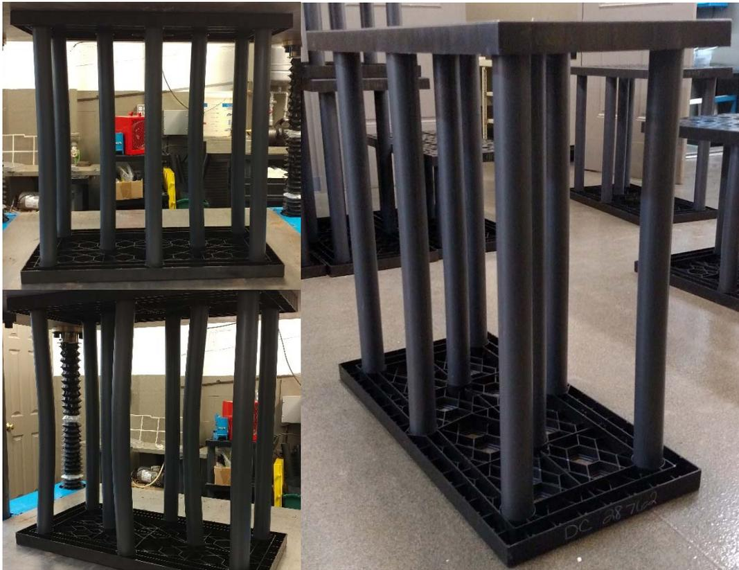
Figure 7 - 36" Module at 20,000 lbs., at completion, and after removal from steel press
